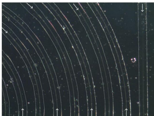
Figure 3. The spiral chip. a) Focused 8 \mu\text{m} particles in a flow rate of 100 \mu\text{L}/\text{min} . b) Focused 8 \mu\text{m} particles in a flow rate of 500 \mu\text{L}/\text{min} . The shift of the focused band towards the spiral centre can be seen. The arrows indicate the flow direction. A downwards flow direction in the figure is flow moving to the spiral centre and upwards flow direction is flow moving from the spiral centre.
