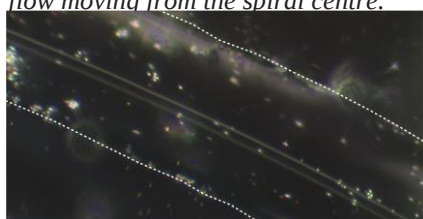
Figure 4. The formation of two bands in the spiral channel when focusing 8 \mu\text{m} particles in a flow rate of 500 \mu\text{L}/\text{min} . The chip is viewed tilted to visualize the two bands.
