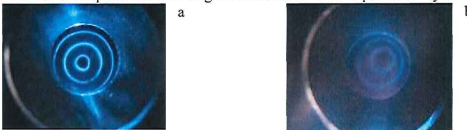
Figure 3 Two aerosol emerging from a tube vibrating to produce the same resonance in the cavity. a) water droplets \sim 5 \mu\text{m} diameter, b) smoke particles \sim 2 \mu\text{m} diameter.
