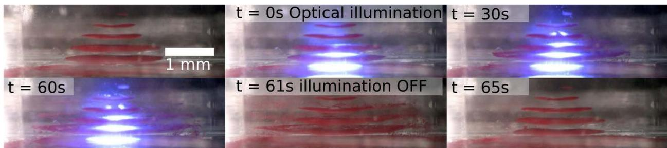
**1:** Examples of the optical ejection of particles coupled with multi-node acoustic levitation. After acoustic levitation, then the optical illumination ejects the particles from the monolayer successively from the first to the last aggregate of the acoustic levitation column.
