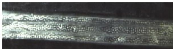
Figure 4: Bridge depth 0.2 mm ( $\sim\lambda/7$ ). An array of small clumps form on the polystyrene surface.
