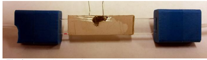
Fig. 2. Flow cell made of a commercial rectangular glass capillary with PDMS connectors and PTFE tubing.
