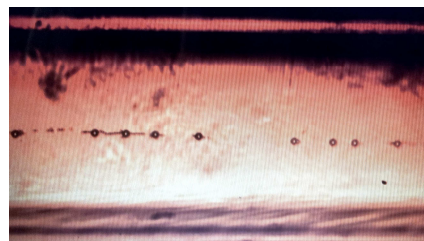
Fig. 1. a) The square capillar with a length l = 40 mm, inner width w = 0.7 mm, and inner height h = 0.7 mm. It is glued to a piezoelectric ceramic pz26 (30.0 mm \times 30 mm \times 1.0 mm) and mounted under the microscope attached to a high-speed CCD camera. The piezo has the dimension. b) Both small and large particles collect almost perfectly aligned at the channel center driven by the primary radiation force, generating a 1D chain along the channel length
